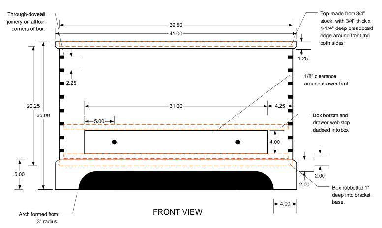
Note: Box is made from 3/4" stock. Bracket base made from 1" stock. Preferred lumber is chery.
